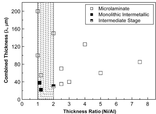
Fig. 3. Diagram summarizing the microstructure type with respect to the thickness and the thickness ratio.
