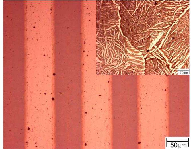
Fig. 2. Microstructures of intermetallic/metal microlaminate (initial  $t_{\text{Ni}} = 100 \mu\text{m}$ ) obtained by reaction synthesis at  $t_{\text{Ni}}/t_{\text{Al}} = 1:1$ . The inset shows a monolithic intermetallic (initial  $t_{\text{Ni}} = 20 \mu\text{m}$ ).
