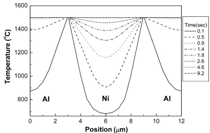
Fig. 5. Transient thermal gradient during the formation of NiAl at  $t_{Ni} = 5 \mu\text{m}$ .
