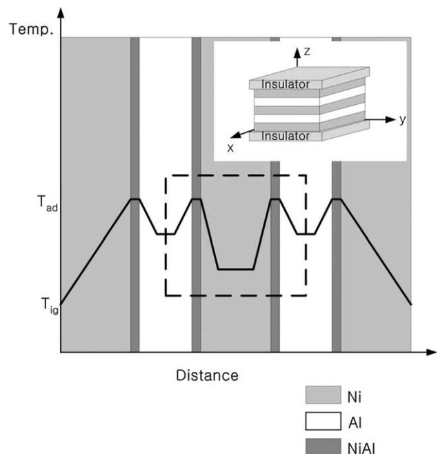
Fig. 1. Sample setup (inset) and schematic  $xz$  or  $yz$  plane used for transient thermal analysis during reaction synthesis of Ni/Al microfoils. Dotted box is symmetric element for finite element modeling.
