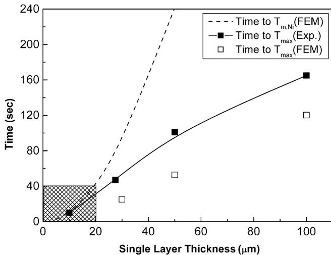
Fig. 7. Comparison of the FEM-simulated and experimental values of the times to  $T_{m,Ni}$  and  $T_{max}$ .
