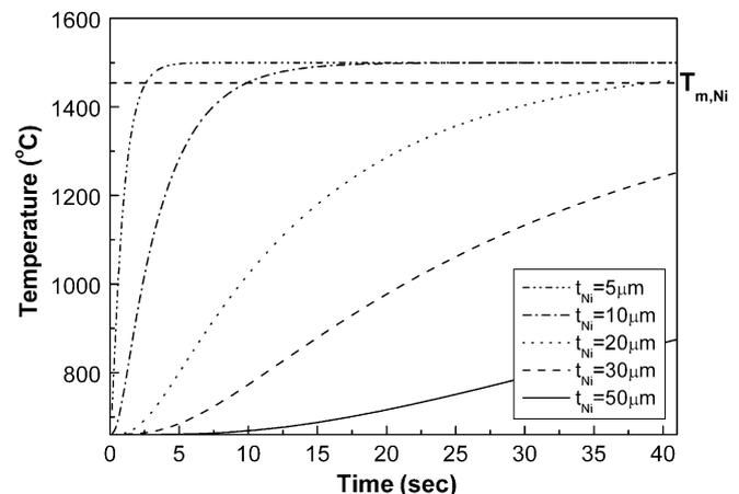
Fig. 6. Time required to arrive at  $T_{m,Ni} = 1455 \text{ }^\circ\text{C}$  as a function of  $t_{Ni}$ .
