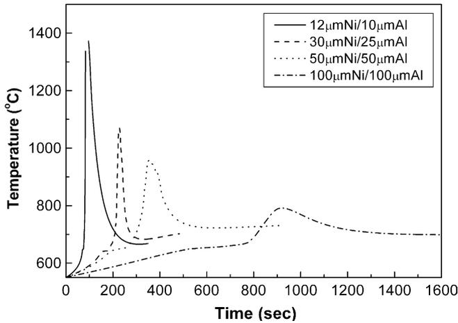
Fig. 4. Time-temperature curves for various combined thicknesses ( $\lambda$ ).
