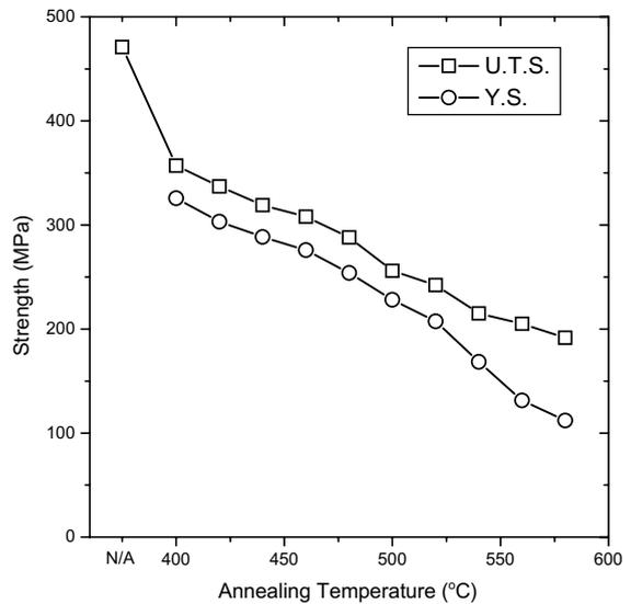
Fig. 2. The variation of yield strength and U.T.S. of ultra-fine Au bonding wires with varying the annealing temperature.
