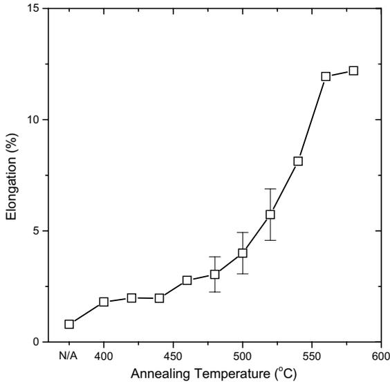
Fig. 3. The variation of elongation of ultra-fine Au bonding wires with varying the annealing temperature.
