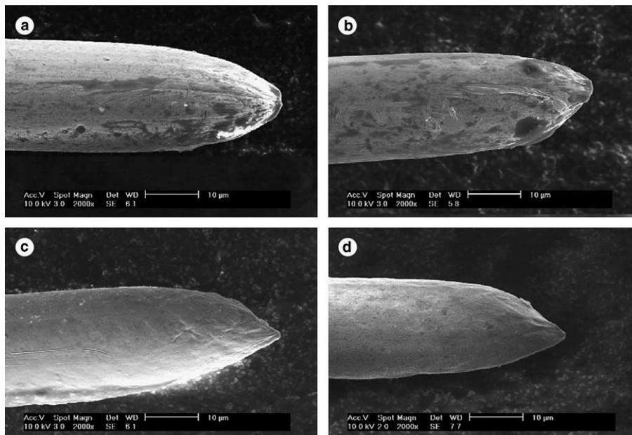
Fig. 9. The shape of fractured end of ultra-fine Au bonding wires after micro-tensile test (a) as-drawn, (b) annealed at 520 °C, (c) annealed at 540 °C and (d) annealed at 580 °C.
