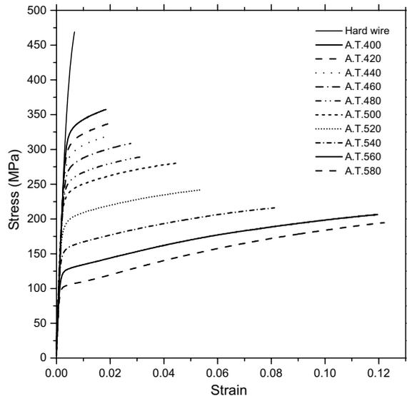
Fig. 1. Stress–strain curves of ultra-fine Au bonding wires obtained by micro-tensile tests.
