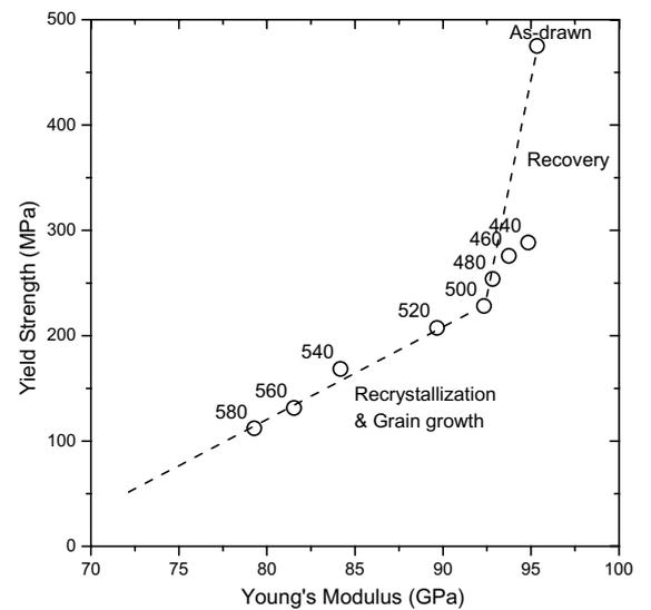
Fig. 6. Plot of yield strength vs. elastic modulus of ultra-fine Au bonding wires.
