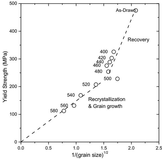
Fig. 11. The variation of yield strength with varying the grain size showing the Hall-Petch type relationship in ultra-fine Au bonding wires.
