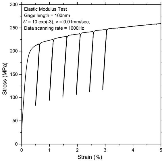
Fig. 4. A series of partial unloading curve during the micro-tensile test of ultra-fine Au bonding wire.
