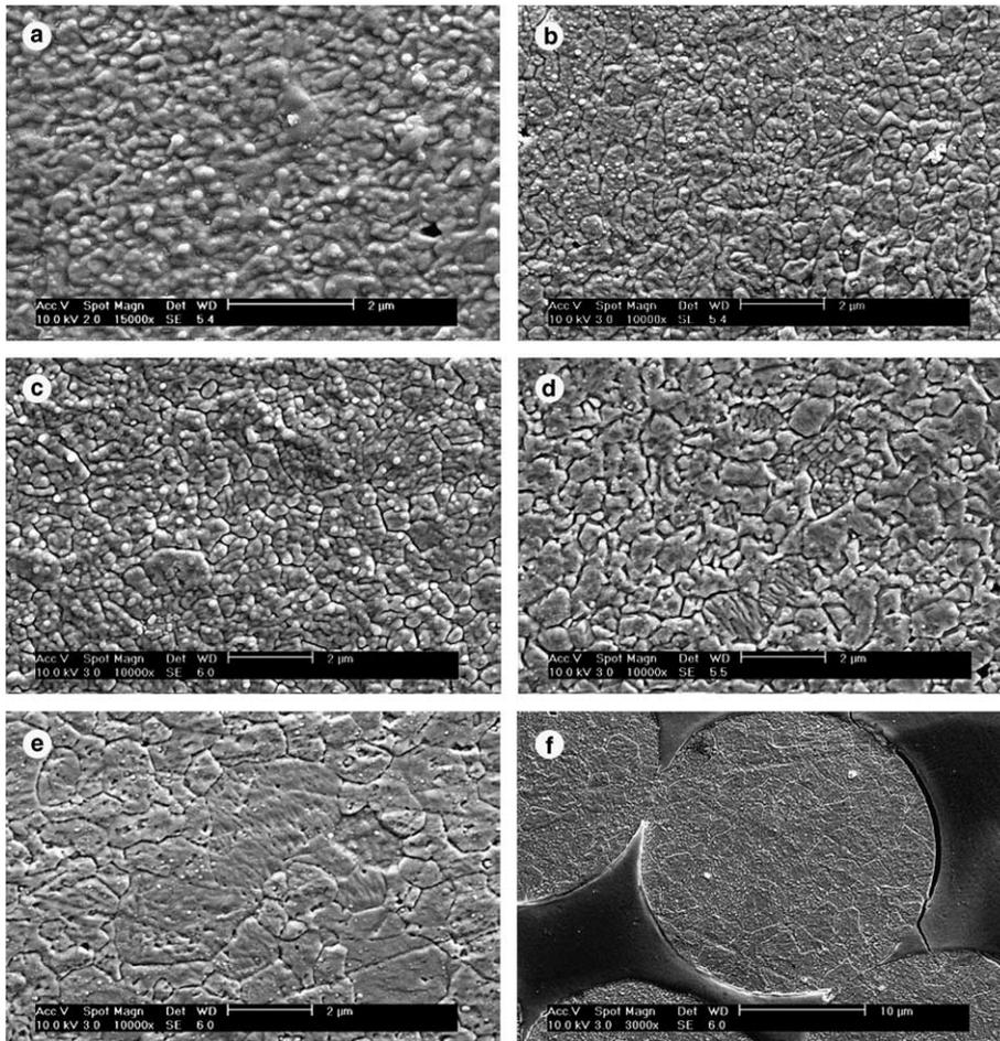
Fig. 7. Microstructure of ultra-fine Au bonding wires (a) as-drawn, (b) annealed at 460 °C, (c) annealed at 500 °C, (d) annealed at 520 °C, (e) annealed at 540 °C and (f) annealed at 580 °C.
