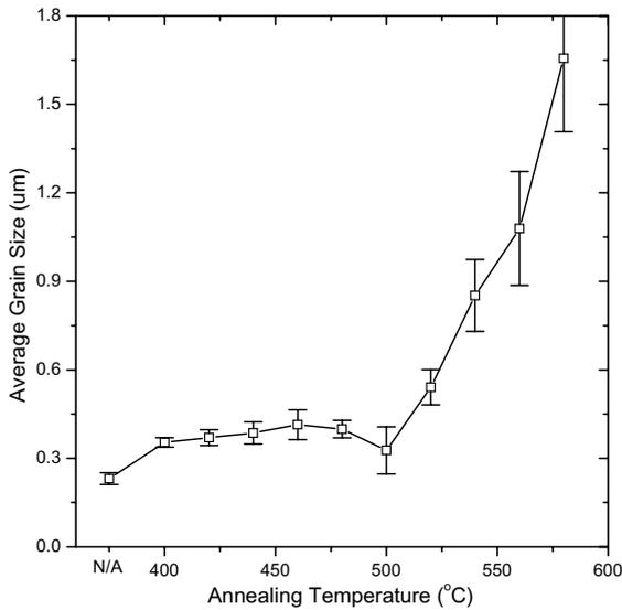
Fig. 8. The variation of average grain size of ultra-fine Au bonding wires with varying the annealing temperature.
