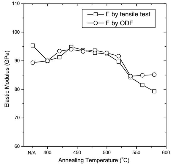
Fig. 5. The variation of measured elastic modulus and predicted elastic modulus with varying the annealing temperature.
