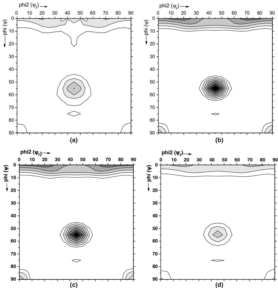
Fig. 10. Orientation distribution function characterized from X-ray diffraction of ultra-fine Au bonding wires (a) as-drawn, (b) annealed at 500 °C, (c) annealed at 520 °C and (d) annealed at 540 °C.
