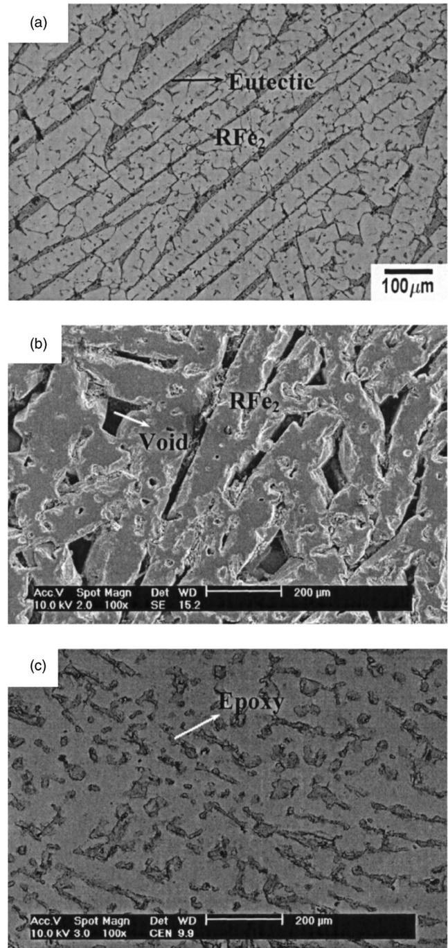
FIG. 1. Transverse sections for (a) the as-grown crystal, (b) the preform before making the composite, and (c) the filled composite with a composition of  $\text{Tb}_{0.33}\text{Dy}_{0.67}\text{Fe}_{1.36}$  observed under optical or scanning electron microscope micrograph fitted with a backscattered electron.
