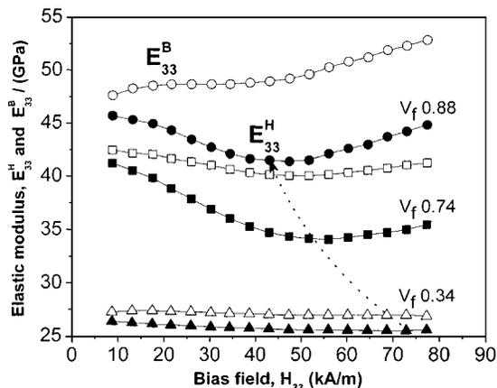
FIG. 3. Variation of  $E_{33}^H$  as a function of a bias field of filled composites with an RFe<sub>2</sub> volume fraction in the range of 0.34 to 0.88.
