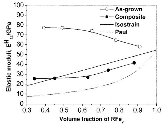
FIG. 4. Dependence of the minima of the  $E_{33}^H$  on the RFe<sub>2</sub> volume fraction in as-grown crystals and filled composites. The solid line was calculated by assuming an isostrain condition of  $E_{epoxy}$ =3 GPa, and  $E_{RFe_2}$ =54.1 GPa; the dotted line is calculated by Paul's formula. (see Ref. 18).
