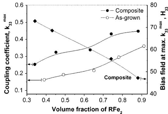
FIG. 6. The maximum coupling coefficient  $k_{33}^{\max}$  and the bias field showing  $k_{33}^{\max}$  as a function of the RFe<sub>2</sub> volume fraction for the as-grown crystals and filled composites.
