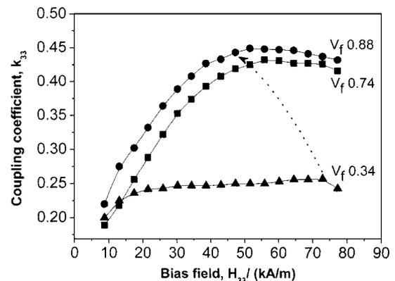
FIG. 5. The magnetomechanical coupling coefficient  $k_{33}$  as a function of the bias field for filled composites with RFe<sub>2</sub> volume fraction values ranging from 0.34 to 0.88.
