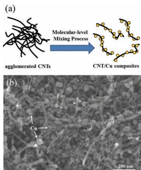
**Figure 1.** (a) Schematic illustration of CNT/Cu composite powders and (b) SEM micrograph of CNT/Cu composite powders.
