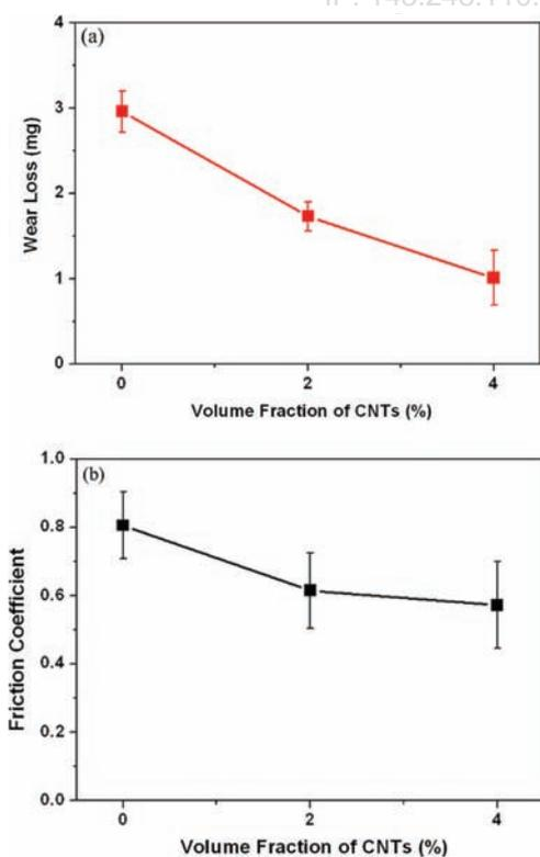
**Figure 5.** (a) The variation of wear loss of CNT/Al-Cu composite with the volume fraction of CNTs and (b) the variation of friction coefficient of CNT/Al-Cu composites with the volume fraction of CNTs.
