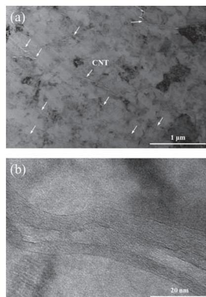
**Figure 3.** (a) TEM micrographs of 4 vol.% of hot extruded CNT/Al–Cu composites and (b) its high magnification image.
