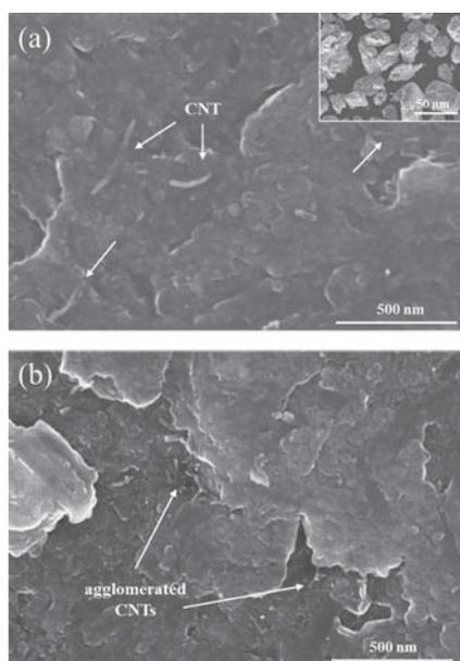
**Figure 2.** (a) SEM micrograph of CNT/Al–Cu composite powders and (b) SEM micrograph of CNT/Al powders from pristine CNTs.
