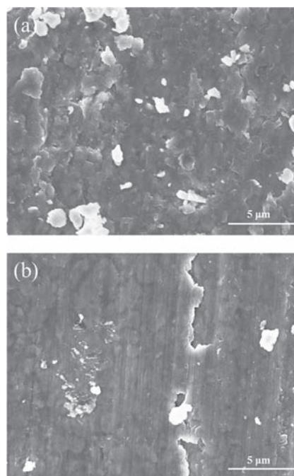
**Figure 6.** (a) SEM micrograph of worn surface of Al-Cu and (b) SEM micrograph of worn surface of CNT/Al-Cu composites.
