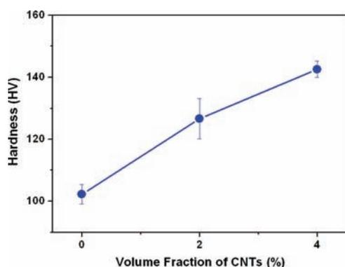
**Figure 4.** The variation of Vickers hardness of CNT/Al-Cu composite with the volume fraction of CNTs.
