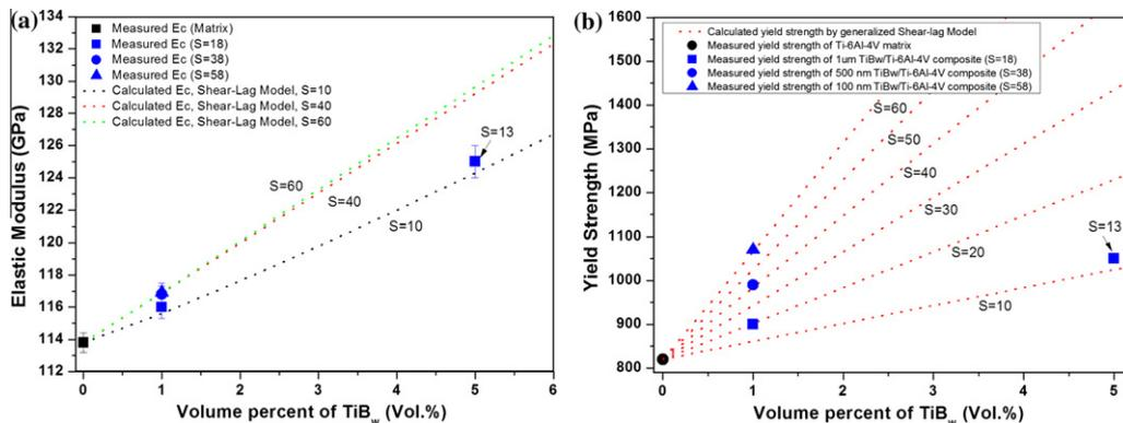
Figure 2. Comparison between the measured and calculated mechanical properties for (a) the elastic moduli of 1 and 5 vol.% TiB<sub>w</sub>/Ti-6Al-4V composites with different  $S$  of TiB<sub>w</sub> and (b) the yield strengths of 1 and 5 vol.% TiB<sub>w</sub>/Ti-6Al-4V composites for aspect ratios from 10 to 60 (dotted lines).
