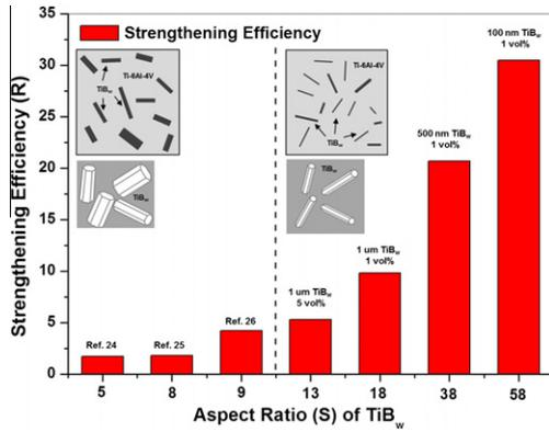
**Figure 3.** Comparison of strengthening efficiencies of  $TiB_w/Ti-6Al-4V$  composites with  $TiB_w$  of different aspect ratios.
